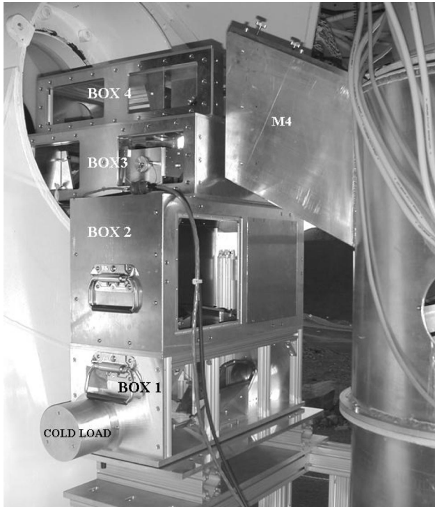
Fig. 5. Modular design of SHARP. The components in each box are: Box 1—P3h/v (cold load mirrors), Gh/v, F4, and BC; Box 2—P2h/v and F3h/v; Box 3—F1, HWP, XG, and F2h/v; and Box 4—P1 and F5.
