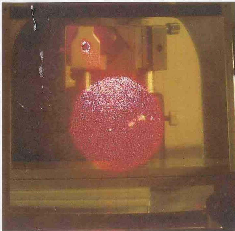
Fig.5 The F12 beam is focused on combiner screen.
