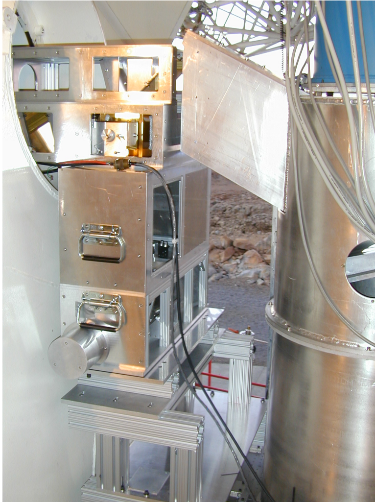
Figure 5.2. The SHARP Polarimeter at the Caltech Submillimeter Observatory (CSO). SHARP consists of four boxes that are mounted at the Nasmyth focus of the telescope. Light comes in through the elevation bearing (from the top left in this photo) into the top box, where it is sent down into the optics path. These optics split the light into orthogonal polarizations and add a linear displacement between the two beams, then sends the light into the SHARC-II camera (located at the top right of this photo).
