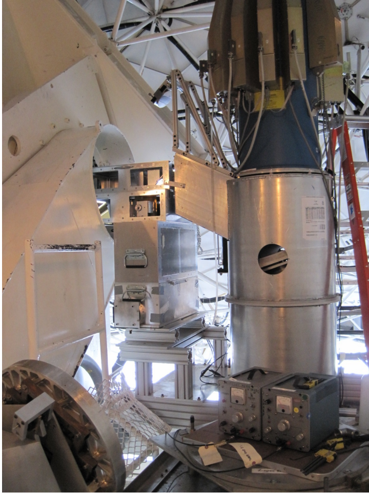
Figure 1: SHARP (stack of boxes at center) and the SHARC-II (cylindrical tower at right) at the CSO.
